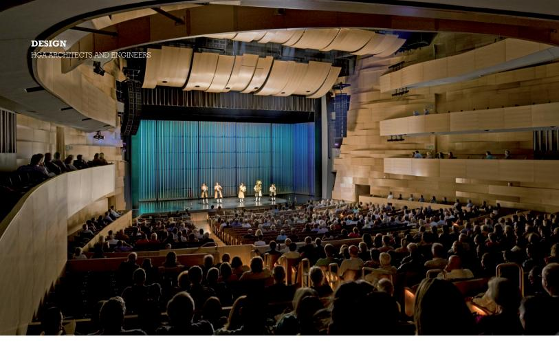
semi-trucks. The stage, 35m-wide and 15m-deep, has an adjustable proscenium frame and 60 manually controlled line sets for stage scenery, draperies and lighting. An easily accessible grid iron is 23m above the stage and the sprung wood floor has a  $4 \times 8m$  modular structurally framed trap. The 636 theatrical lighting circuits can be individually controlled by computer or remote touchscreen panels.
