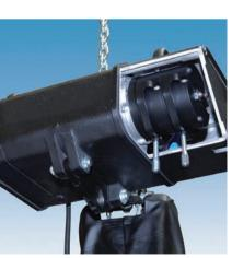
Chain hoist with double brake from the ROBA-secustop series
