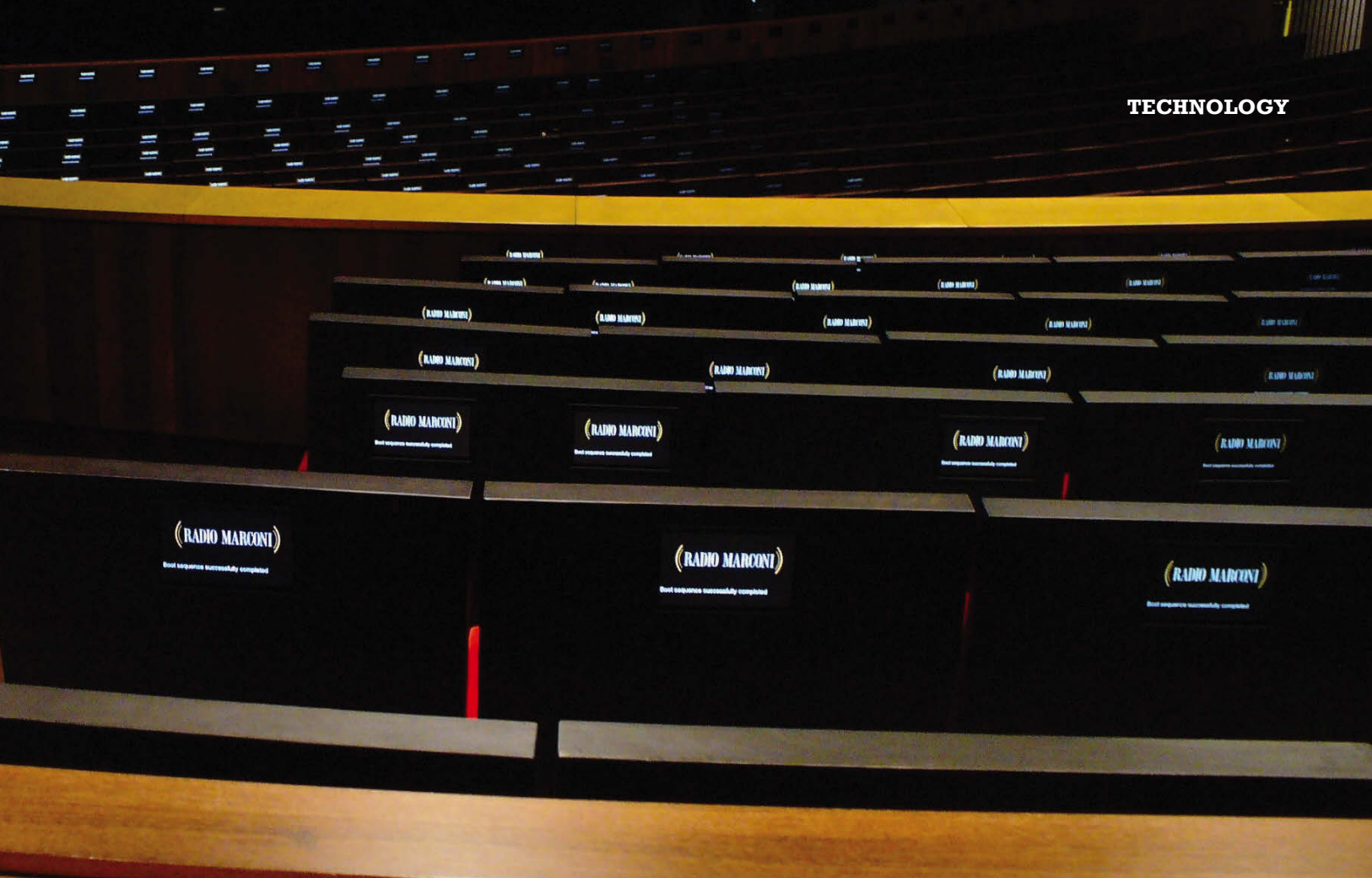
(Above) Screens are subtly integrated into the seat backs (Below, clockwise from left) The theatre information service: welcome screen, opera libretto, performer information and restaurant reservations
