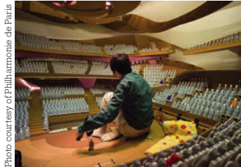
(Above) Large-scale acoustical models offer what architect Jean Nouvel says are excellent listening conditions, providing information that computer simulation cannot (Top) The large auditorium can adapt physically and acoustically to different musical styles
