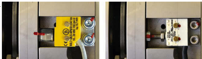
Above: The contactless release monitoring with inductive proximity switch (left) and the release monitoring with microswitch (right) have the same installation dimensions and are interchangeable Below: In the stage drives of the Theatre and Philharmonic Essen, stage brakes with Mayr's contactless release monitoring guarantee top operational reliability
